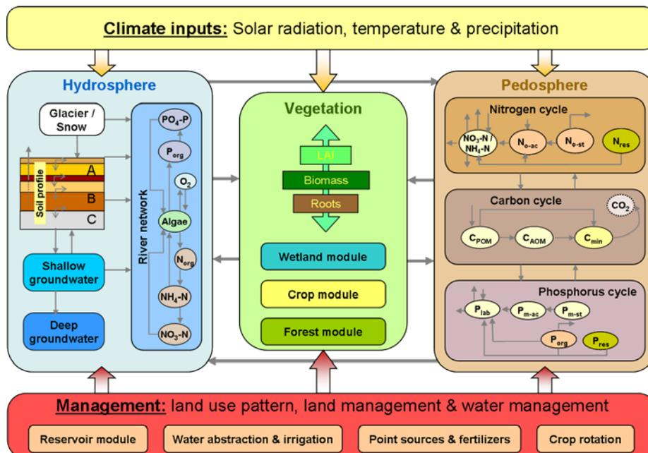
Figure 16: SWIM (Soil and Water Integrated Model)
